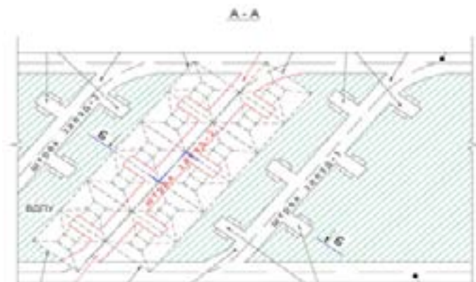
Figure 1a. The plan of the proposed block caving geotechnology with the new modification of the process chart for chromite mining in combination with vibratory ore drawing under the artificial stope sill at deep levels of the mine.
